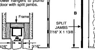
5. Fasten bottom door guides so that door stays in center of pocket, yet travels easily without binding.
